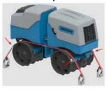
If the machine is supposed to be strapped down, this must be done via the drums. To prevent them from sustaining damage, the scrapers must either be dismounted or supported on the drums with the help of wooden wedges.
